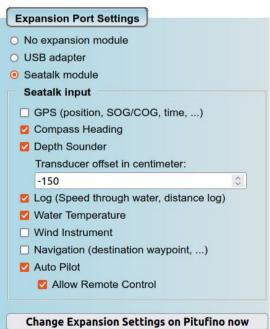
supported without a module (see section 1.2). The settings include an input filter and a separate checkbox whether Pitufino is allowed to remote-control the autopilot. Note, selected navigation data in the input filter is sent to TCP/UDP streams as well as converted to NMEA2000 and sent to web apps. Also the function of the relay can be selected here, either as an external alarm or as a general switch that can be controlled from Pitufino's web apps.
